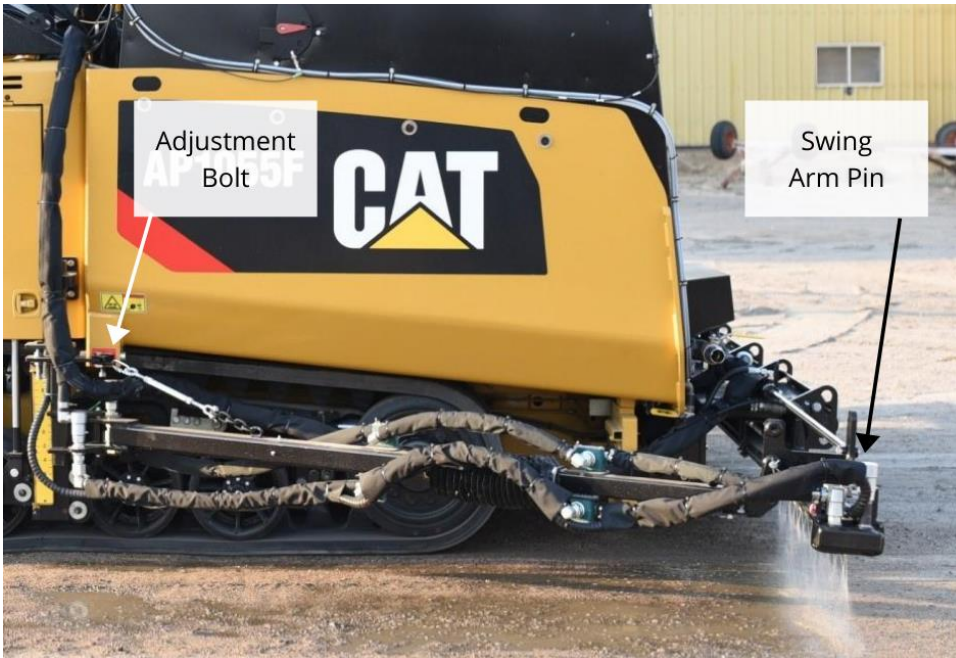
Figure 11: Swing arm height adjustment points
