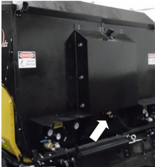
Figure 49: Clean out tank manual ball valve
