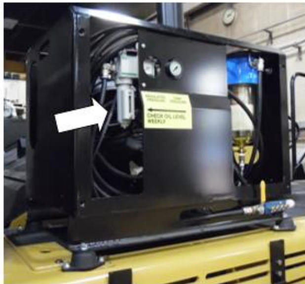
Figure 54: Air lubricator sight gauge location.
