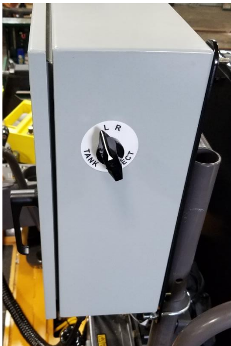
Figure 27: Tank select switch
