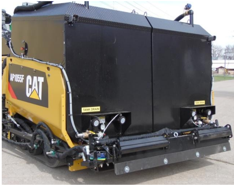
Figure 5: Front spray bar housing, telescoping spray bars retracted
