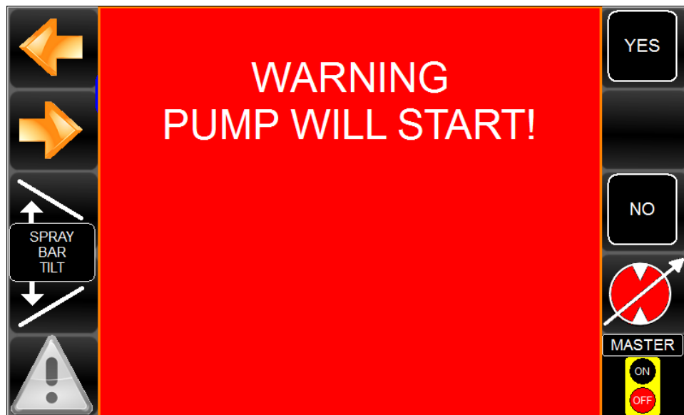
Figure 33: Pump will start warning screen
