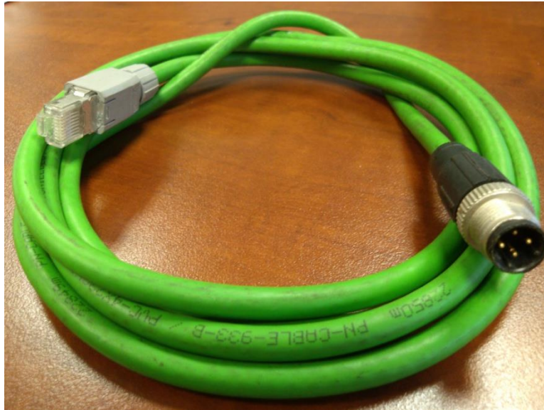
Figure 58: Ethernet cable 1DX10880
