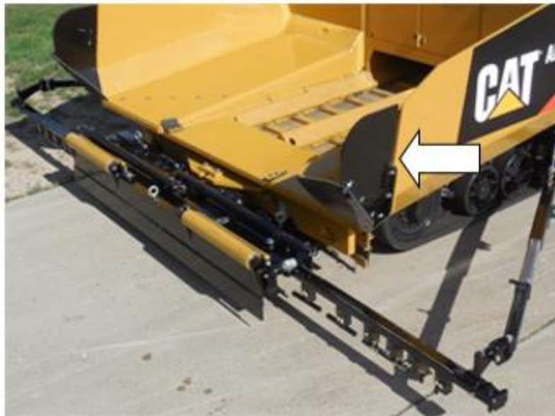
Figure 15: Asphalt hopper extensions
