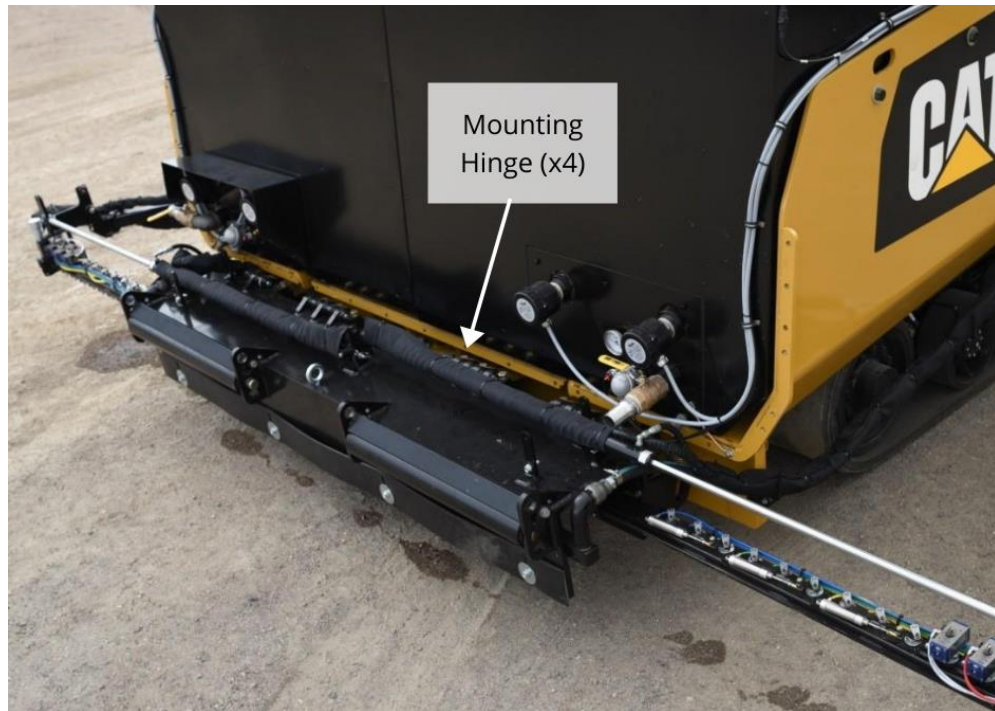
Figure 10: Front spray bar mounting hinges with spacers underneath
