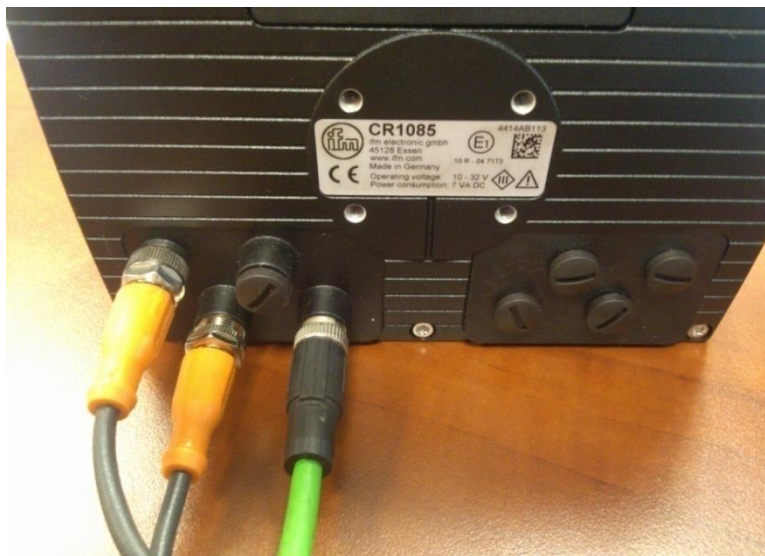
Figure 59: Displays screen unit back side showing the Ethernet cable connection
