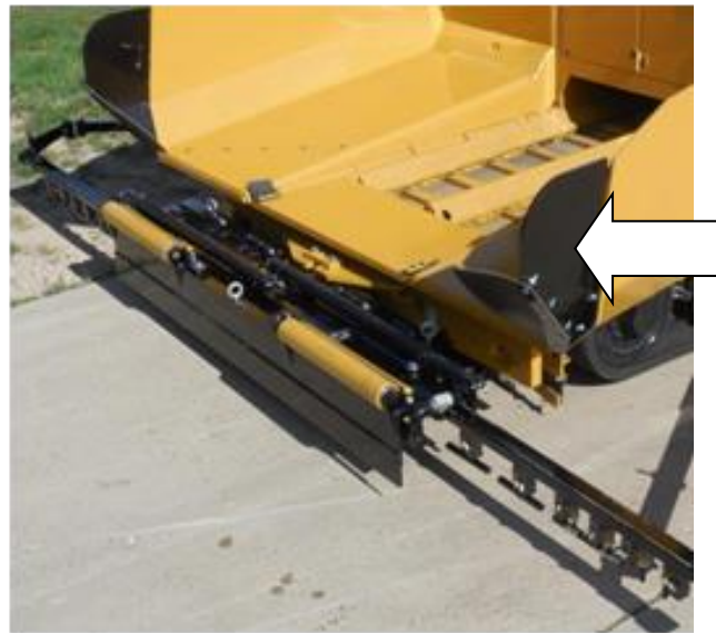
Figure 16: Asphalt hopper extensions
