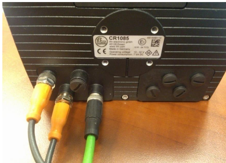
Figure 51: Displays screen unit back side showing the Ethernet cable connection
