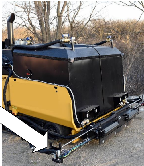
Figure 6: Front spray bar housing, telescoping spray bars extended
