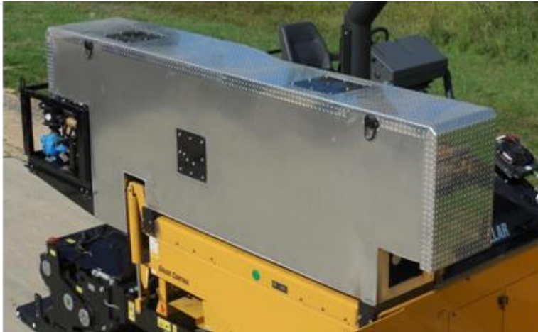
Figure 3: Emulsion tank, deck mounted
