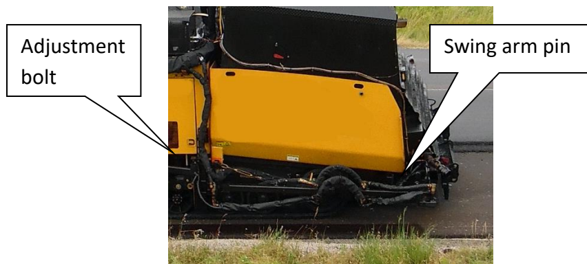
Figure 12: Swing arm height adjustment points
